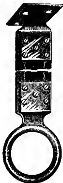
Fig. 4224. UPPER-BERTH SAFETY-ROPE HANGER.
